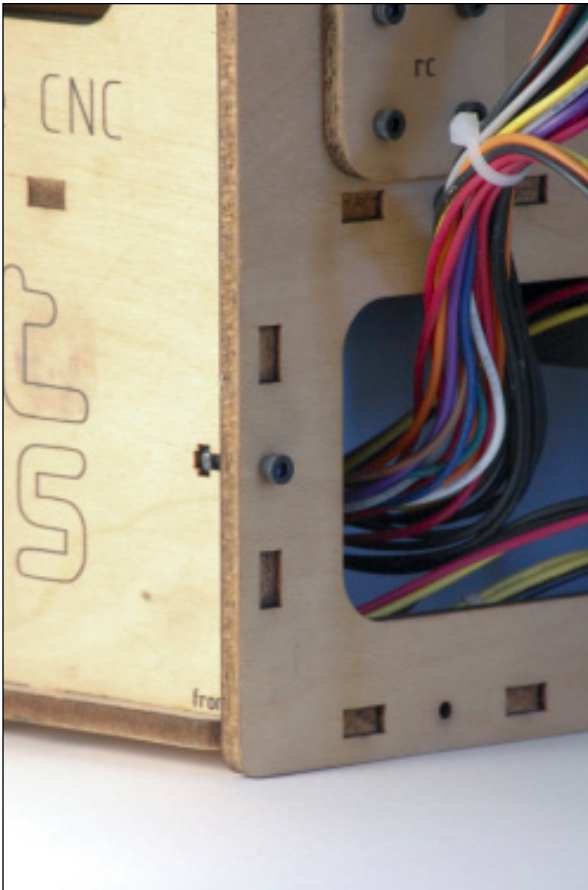
Bolted tenon or T-slot joint.
