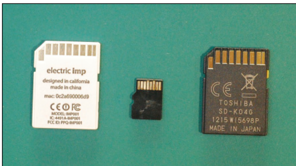
The rear of (from left to right): an Electric Imp, a micro SD card, an SD card.
