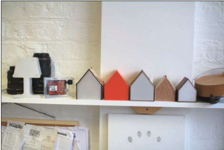
The evolving design for the Good Night Lamp (from left to right): original design; functional mockup; redesign mockup; redesign functional prototypes (orange and wood/acrylic); revised size mockup; revised size functional prototype.
